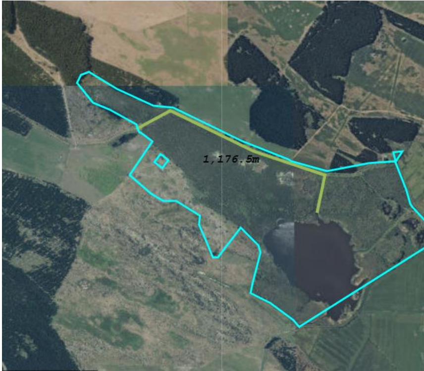
Figure 10: Pukepuke Lagoon perimeter drain
